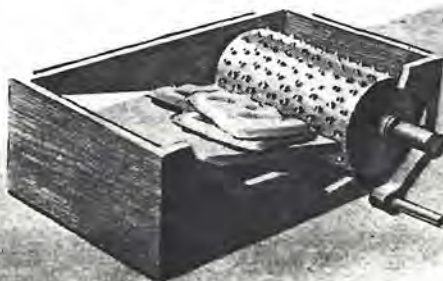
CRACKER MILL provided flour for making pies. Crackers were pressed against a rotating cylinder on which teeth had been raised with a nail. Flour dropped into the bottom section.
