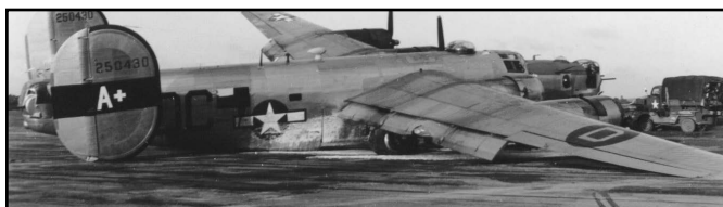
This photo of #42-50430, Old Standby , was taken after it snapped its landing gear while returning from the mission on 18 Sep 1944. It shows the black Circle D on the right wing and the new design for the tail fins.
