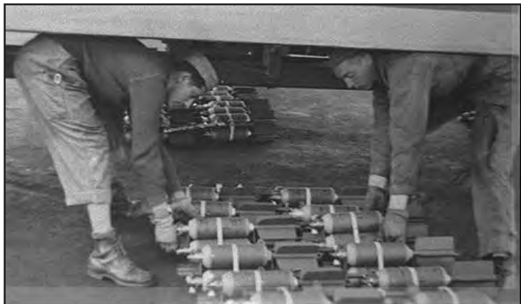
578th Sqdn personnel at work. At left, Cpls Gaetano (Guy) Spinelli and Ken O'Boyle prepare to hoist fragmentation bombs into a bomb bay for D-Day. At right, ordnance personnel move a dolly and bomb to the bomb bay.
