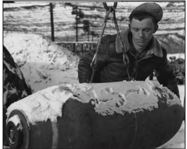
Moving bombs at the bomb dump. Note the camouflage netting overhead and the two lugs on top of the bomb to which the shackle would be attached.
