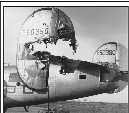
#42-50390 after being strafed by a German fighter pilot on 20 Mar 1945. The ship was repaired and flew back to the US in June.
