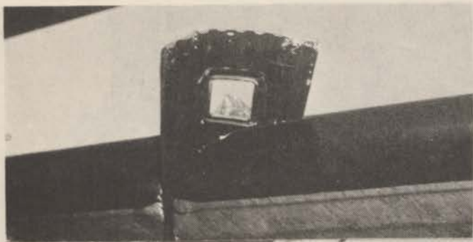
Aircraft #314 lands with section of nose turret door imbedded in stablizer.
