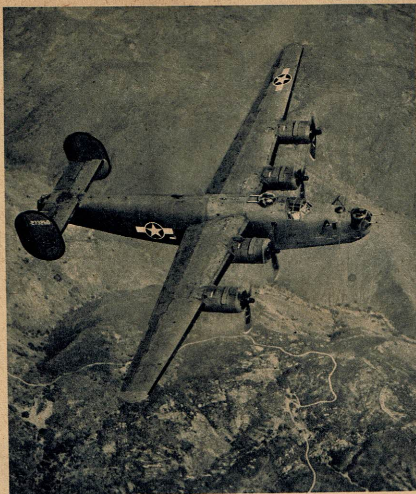
SIZE AND TAPERING OF DAVIS WING are so calculated that the B-24 can carry a greater load farther and faster than any other bomber.
