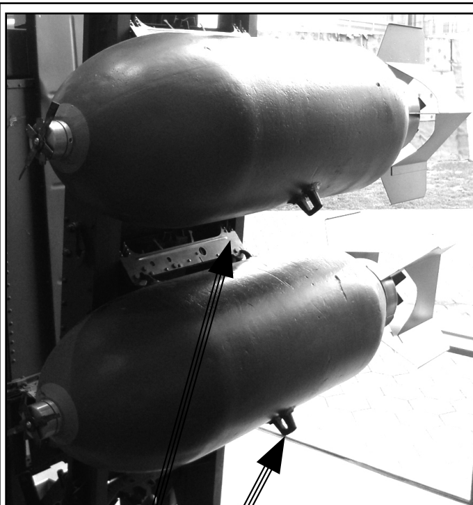
Above: a bomb rack on display in the US Freedom Pavilion. A metal clip (the shackle) was clamped onto two lugs at the top of a bomb (visible at the bottom of these bombs is the one lug used on US Navy planes). The shackle was then hooked onto the bomb rack. When the bomb was released, its shackle disengaged simultaneously from both lugs. A bomb was "hung up" when one end did not completely separate from the shackle. An airman then had to step out on the narrow catwalk in the bomb bay (without a parachute—as he wouldn't fit if he wore one—using a portable oxygen bottle or holding his breath, and at bombing altitude) and kick the bomb loose.
