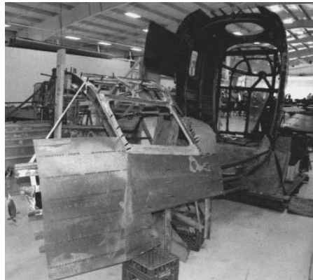
Work under way: Cockpit forward section from RB-24A 40-239. MICHAEL O'LEARY
