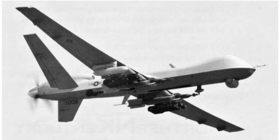
The Reaper is 36 feet long, has a wingspan of 20 feet, a normal service ceiling of 50,000 feet, at speeds of up to 250 mph, and can stay in the air for up to 28 hours. Unit cost is around $8,000,000.
