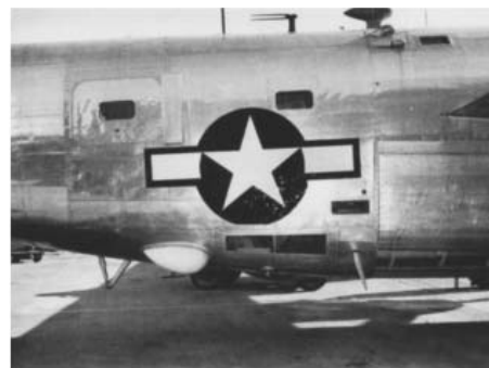
Detail of an unknown B-24 "Ferret." Some of the modifications visible include additional windows and antennas for the APR-4 and APR-5 receivers.
