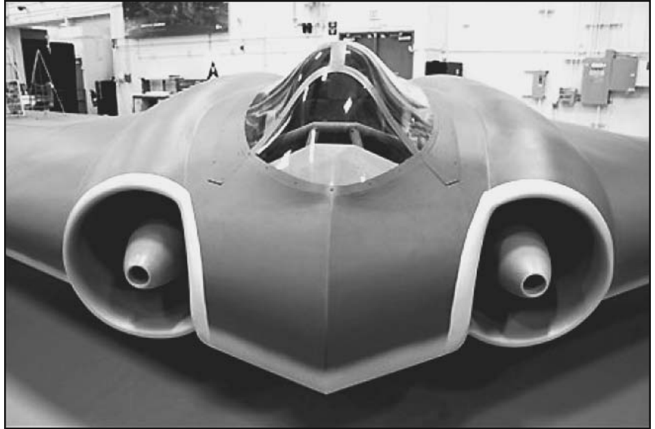
The recessed engines of Hitler's stealth fighter (replica shown at a California facility in late 2008) would have helped the plane avoid radar detection.
