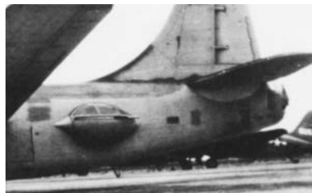
Finally – the Navy installed two waist gun turrets on their PB4Y-2s — their modified version of the Liberator which they renamed the “Privateer.” They used it in late 1944 and 1945 for submarine patrol.
