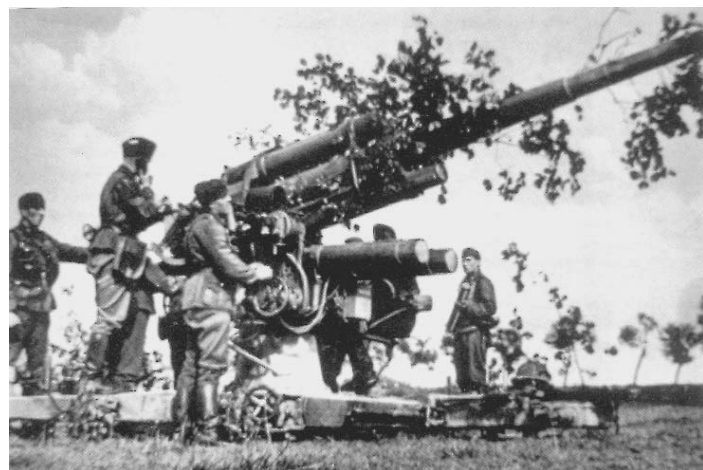
An 88mm flak cannon set up to fire at aircraft. The cruciform mount has been lowered to the ground and leveled. The wheel bogies have been removed. When used as an anti-tank weapon the gunners were protected by forward facing armor plate.
