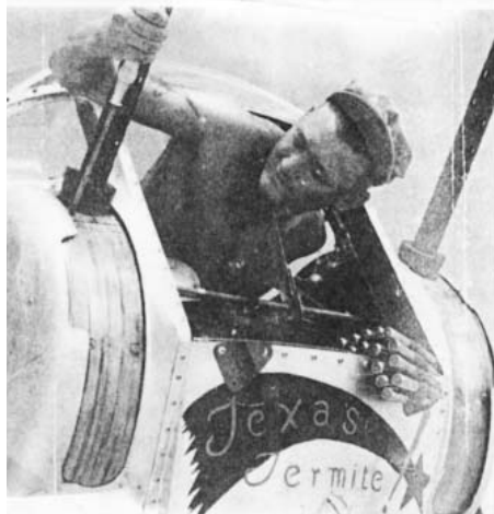
This armorer was making adjustments to the ammunition chute assembly on an MPC tail and nose turret. Note the difference in glazing when compared with the A-6 turret.
