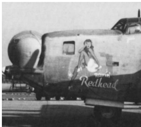
The Navy installed an Erco bow turret on the B-24D's it got from the USAAF in 1943.
