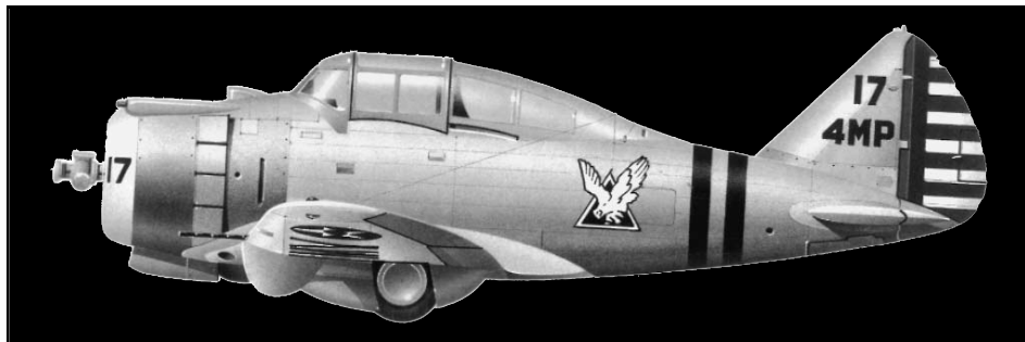
A predecessor to the P-47, the P-35 was the first all-metal monoplane with an enclosed cockpit. The long-range, extremely fast escort fighter won three consecutive Bendix Air Races in the late 1930s.
