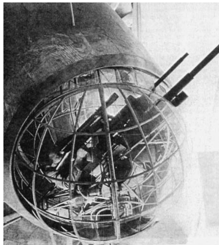
Hydraulically-driven nose turret with cannon and machine gun.
