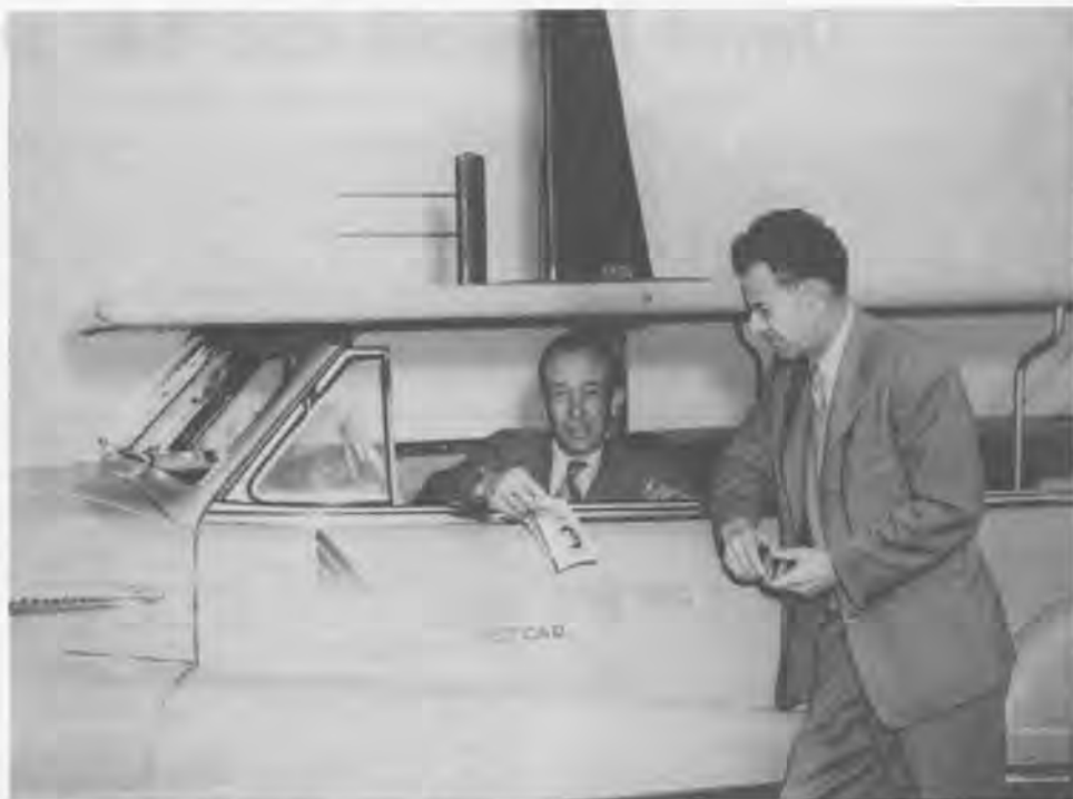
Davis continued to use the automobile as his airfoil testing device during the post-Consolidated wartime period. This is the "Davis Airfoils Test Car," a 1942 Buick convertible with a removable platform for mounting instrumentation and the wing section under test. Person in car is Leland Reid; Davis stands alongside. Photo taken in 1943. Note that wing section was mounted vertically. (Courtesy Bob Reid)
